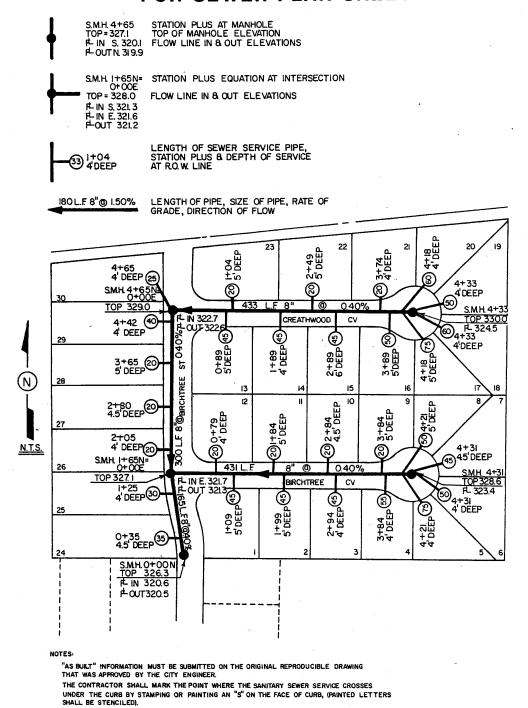
SANITARY SEWER SERVICE LINES SHOULD EXTEND AT LEAST PAST THE RIGHT-OF-WAY LINE IN ALL STANDARD SUBDIVISIONS.
