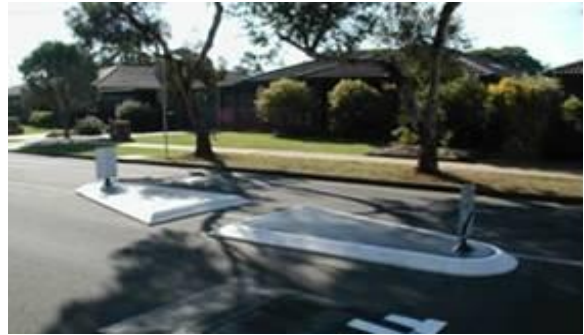
Raised medians reduce the width of the adjacent travel lanes.
