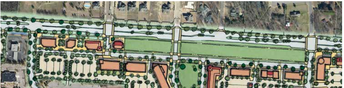
Winchester Road Access – Two full intersections between Tyndale Street and Crestwyn Hills Drive. Second preferred alternative.
