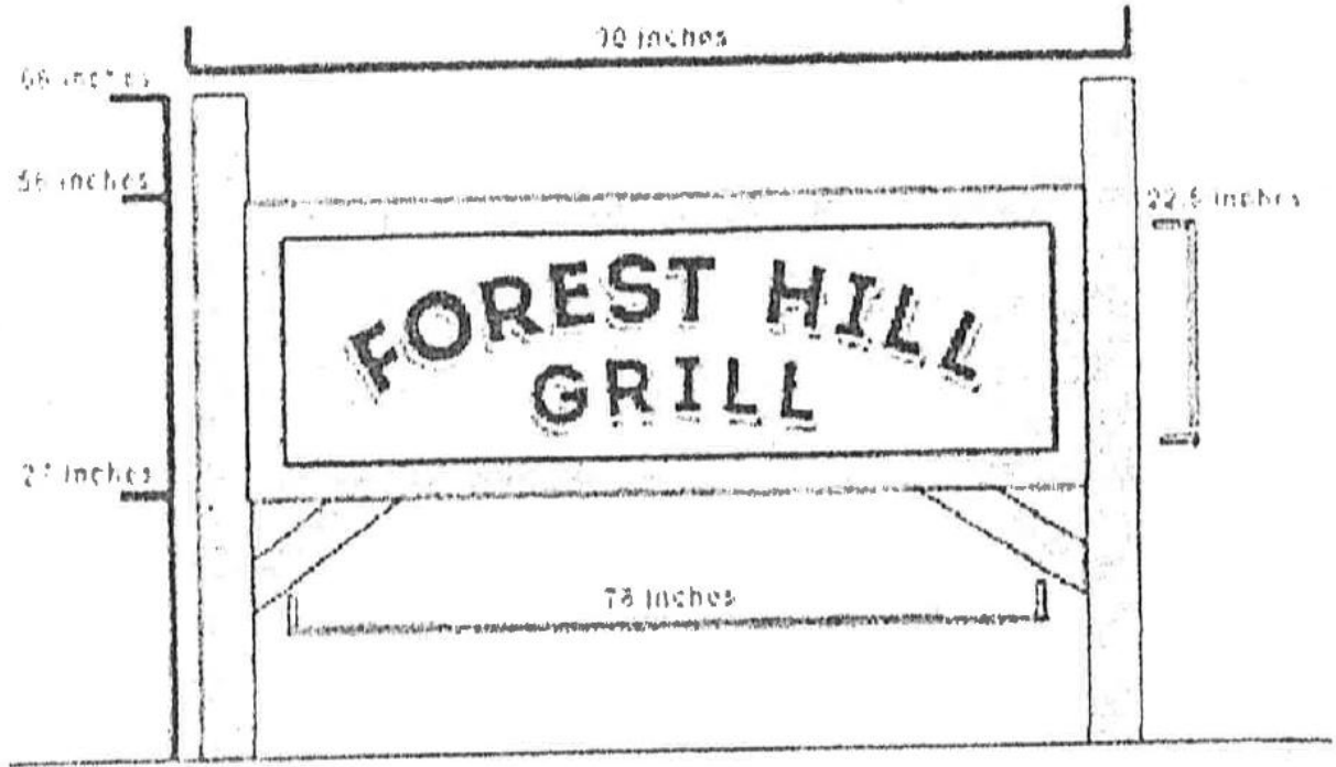
Sign lettering is 3 inches tall. The letters are black on a light grey field.
