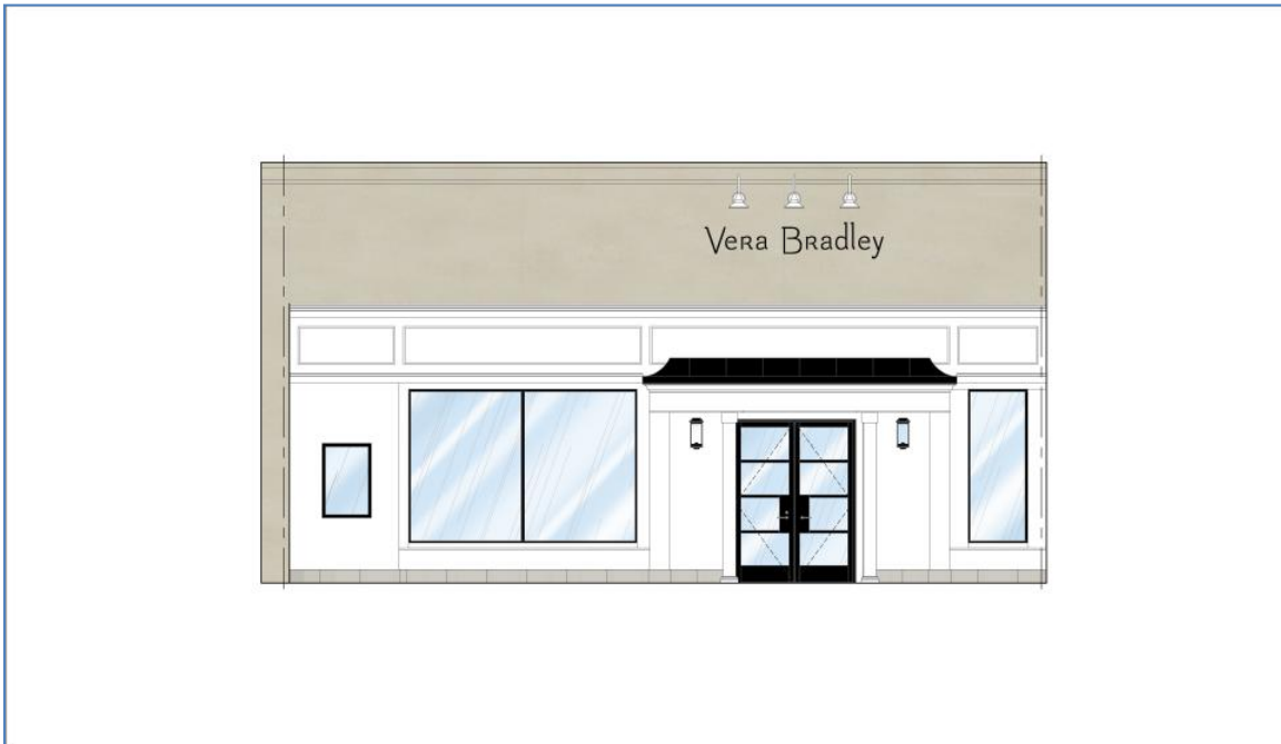
SHOPS AT SADDLE CREEK - GERMANTOWN, TN VERA BRADLEY - PROPOSED STOREFRONT REMODEL ELEVATION SCALE: 1/4" = 1'-0" PROJECT NUMBER: 17158 06/22/17
